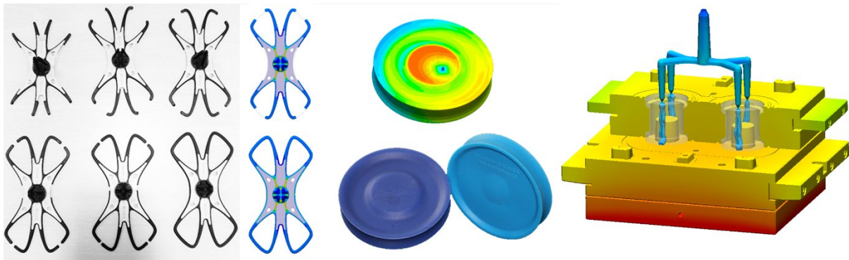
Figure 1 – The different parts can be found simulated as well as in reality on the DKT ("Butterfly", Mini-Frisbee, and vibration dampening part from left to right).
